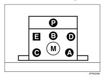
The machine indicator shows the place where the door/units are not closed.
